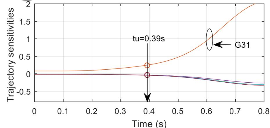
Trajectory sensitivities of synchronous machine's output to OMIB angle
