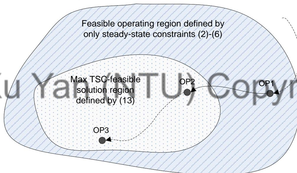
**OP1:** Initial optimal OP determined by a conventional OPF
