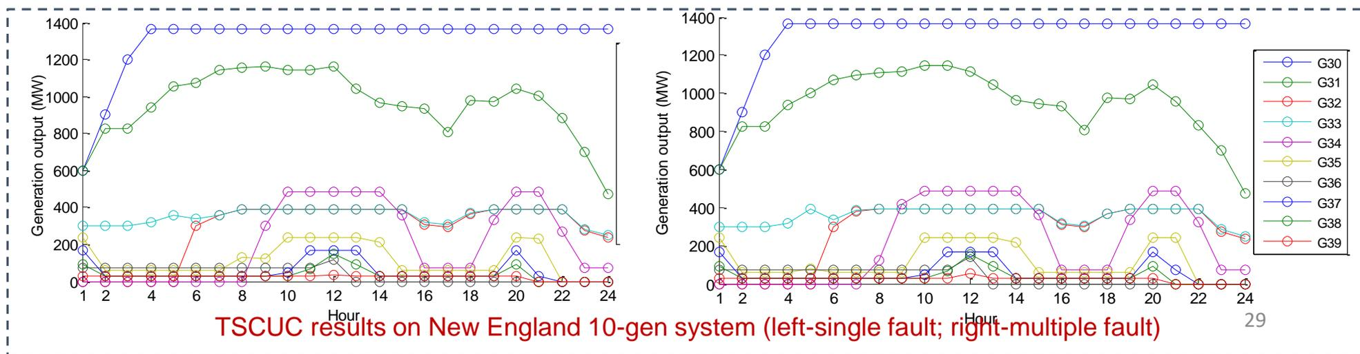
TSCUC results on New England 10-gen system (left-single fault; right-multiple fault)
