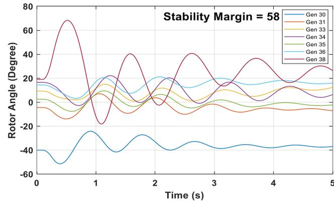
Rotor angle curve under a non-worst case with ELS
