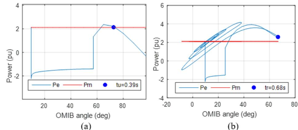
Fig.5  $P_e$ -OMIB angle plane for C1 under  $l_1$ : (a)-unstable (under initial clearing time); (b)-stable (under CCT)
