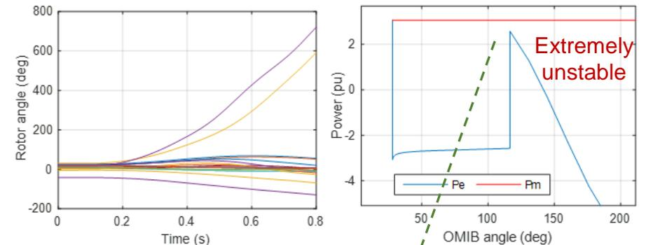
Fig.12 Unstable trajectories for Nordic32 system before dispatch: (a)-multi-machine angle; (b)-Pe-OMIB angle
