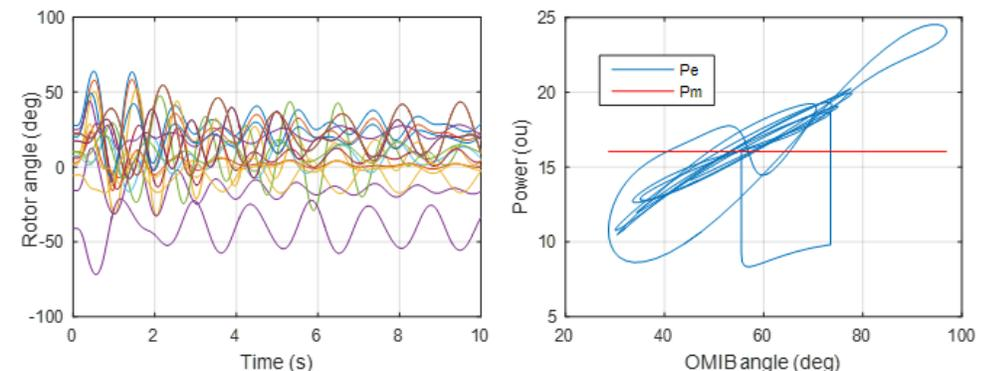
Fig.14 Illustration of stable trajectories for Nordic32 system after dispatch: (a)-multi-machine angle; (b)-Pe-OMIB angle
