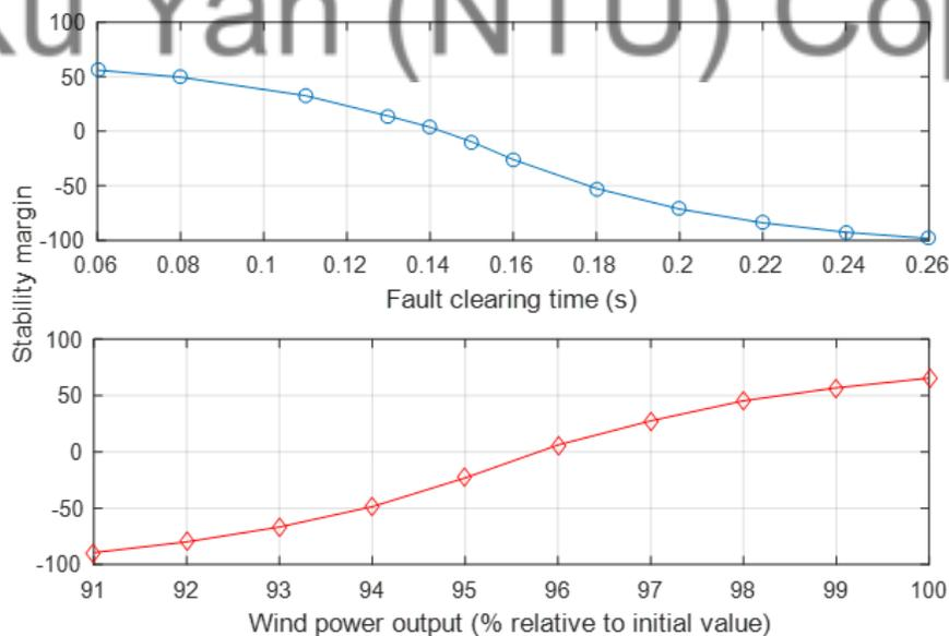
Fig.8 Transient stability margin V.S. key parameters: (a)-fault clearing time; (b)-wind power output
