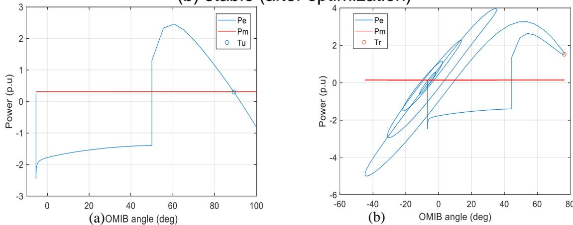
Pe-OMIB angle plane for C1: (a) unstable (before optimization); (b) stable (after optimization)
